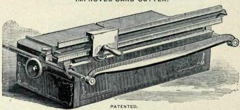
An important feature of this machine is the ease with which the gauge is set to any desired size, from a half-inch to a half-sheet card. This is done by a rack and pinion, accurately cut by special machinery. The position maintained by the gauge is perfectly parallel with the knife. A clamp, conveniently arranged, holds the card firmly, insuring a smooth and true cut.
