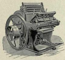
As compared with the old, have heavier shafts, gear-wheels, bridge and platen, greater weight, strength and durability; lighter, smoother and aldutability, lighter, smoother and almost noiseless movement; improved distribution, without any danger of tearing roller; no bridge lugs, no bridge springs, no crescents, and the least possible liability of breakage.
