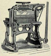
The octagonal stick and recessed sides, admits of passing the stick through the side to its place, and renders it impossible for the stick to be drawn out by the knife, giving sixteen cutting faces on the stick.
