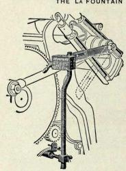
There are no springs to get out of order, and this makes the La Fountain Springless Counter far superior to any other in the market. It is the most simple and durable Counter ever offered to the trade. It registers up to 100,000, and the registering is guaranteed to be perfeet. When the impression is thrown off it will not register.
