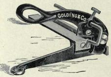
The Nonpareil Lead Cutter is most powerful in the market. Has a long, adjustable bearing for the lever, and both front and back gauges. By pushing the lever, 4-to-pica brass rule can be cut. The lever is held up by a strong spring.
