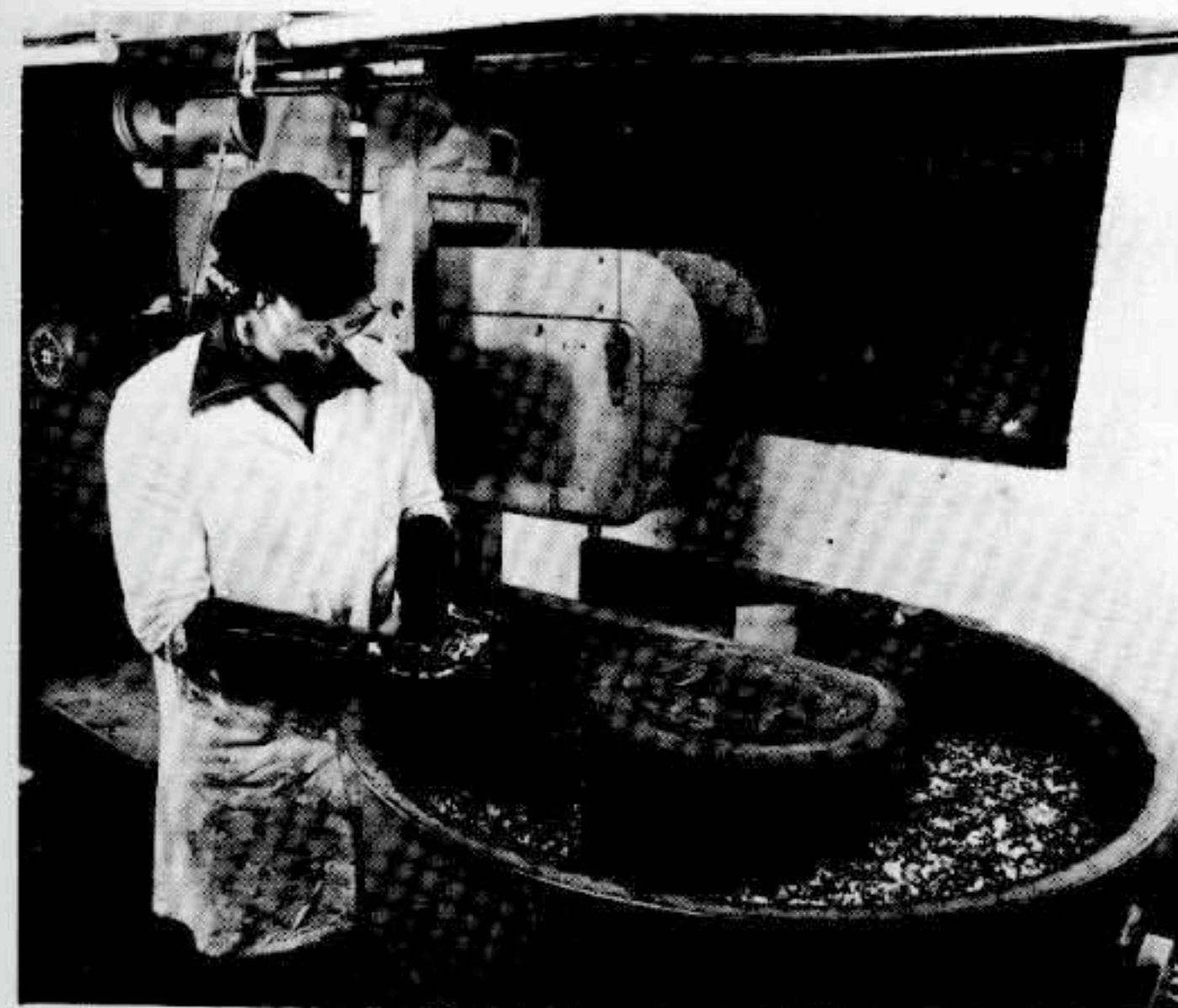
A Vibratory Bowl which takes the place of the old scouring and polishing barrels 1983
