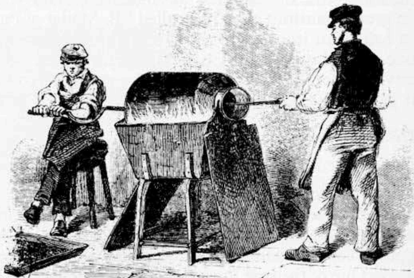
Artists impression of the original method for colouring or bronzing pens. Circa 1850.
