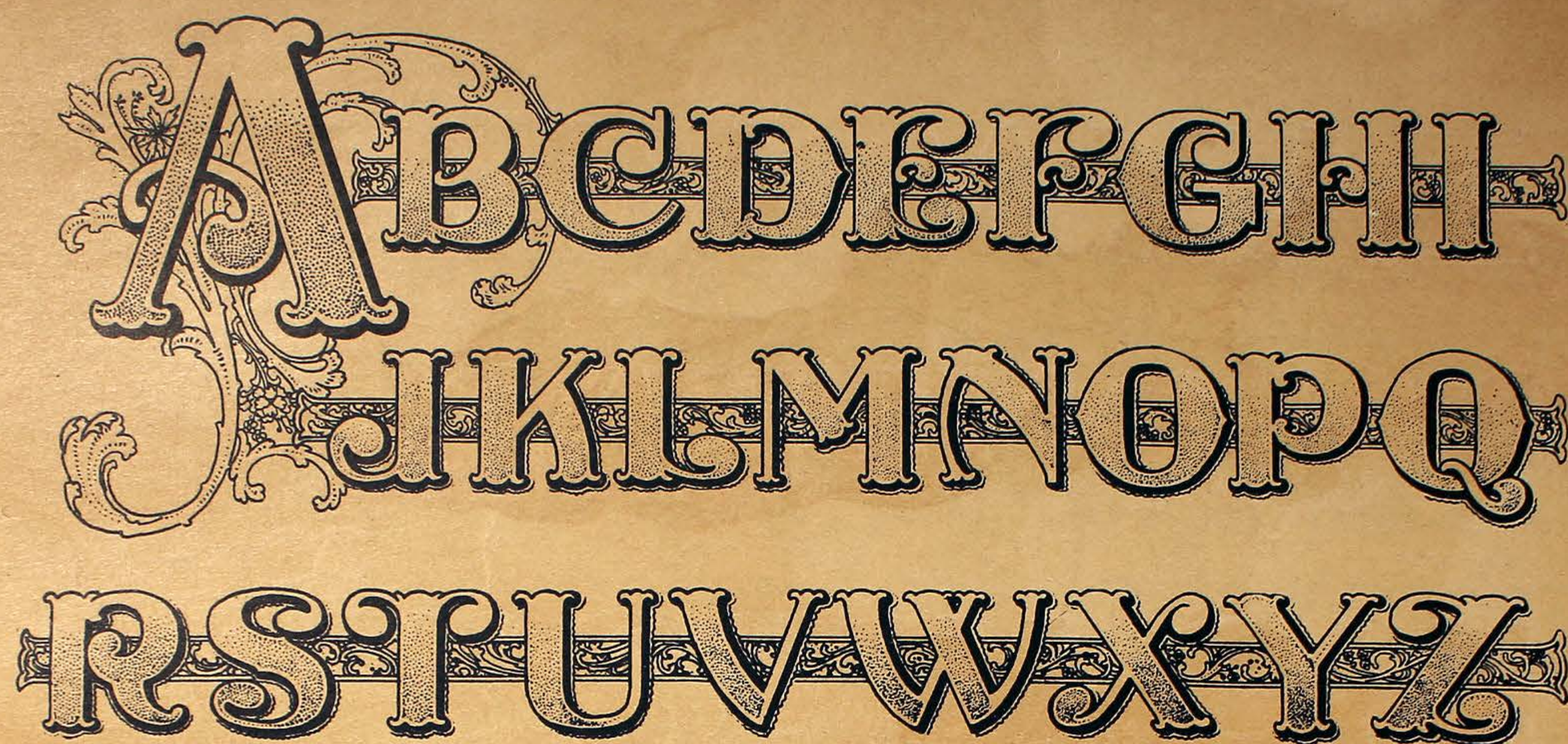
Plate 36. Carefully outline this alphabet with pencil before drawing the heavy outside lines. After all the lines are properly drawn, stipple the letters as indicated. That is done by striking the pen point on the paper.
